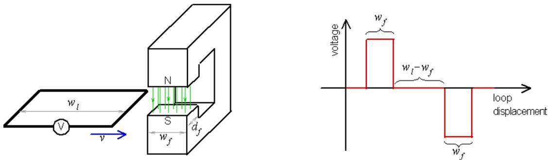
Our exploration setup is depicted above. There is a rectangular wire loop of width ' $w_l$ '. A voltmeter is inserted into the loop to measure the induced voltage. There is also a C-shaped permanent magnet that creates a magnetic field within its gap. The field in the gap has a rectangular cross section (width ' $w_f$ ' and depth ' $d_f$ ', as marked on the picture.)
