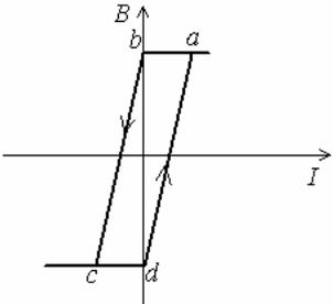
At the beginning we are in the point ‘a’. In the point ‘a’ there is some current in the winding that generates saturation-level magnetic field inside the core.
