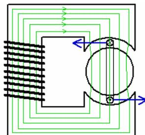
On the picture, the excitation winding creates a weak guidance field that directs the magnetization of the iron frame. The frame has two semi-circular gaps. Within gaps, the
