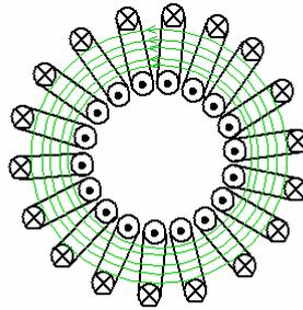
The toroidal coil is an important type of coil where, in an idealistic case, the magnetic field is all confined within toroid volume. There are no magnetic field lines outside the toroid ‘tube’ (not even in the middle of the toroid). To make a toroid coil as close to ideal as possible, the coil should be made from a fine wire and should have dense, evenly spaced wire turns.
