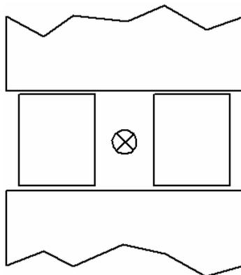
First, let's look at the situation when the electromagnet is switched off, and only the wire generates the magnetic field. As it can be seen on the picture below, the magnetic flux is able to run mostly through iron and so the wire is able to generate relatively strong field within the iron.
