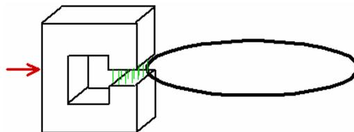
The picture shows an experiment with a conductive wire loop and a C-shaped permanent magnet. We are about to push the magnet rightwards so that its flux crosses the wire and enters the loop. Because the flux through the loop will be increasing, the EMF will be induced along the loop. Because the loop has a small resistance, the current will start flowing in the wire. This current will generate its own magnetic flux of the direction opposite to the magnet's flux.<sup>25</sup>
