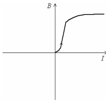
In the above graph, we were increasing the current from zero to some rather high value. As we can see, the generated magnetic field is not linear due to iron nonlinearities. We of
