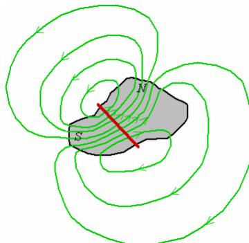
Below is yet another example to help us familiarize with the idea of the magnetic flux. A winding with an iron core is depicted. This particular iron core has an odd, asymmetric three-limbed construction. The winding generates the magnetic flux and the flux ‘moves’
