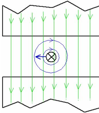
The homogeneous field of the electromagnet is depicted with green lines, and the circular field of the wire is depicted with blue lines. Obviously, there is a force on the wire (blue arrow).
