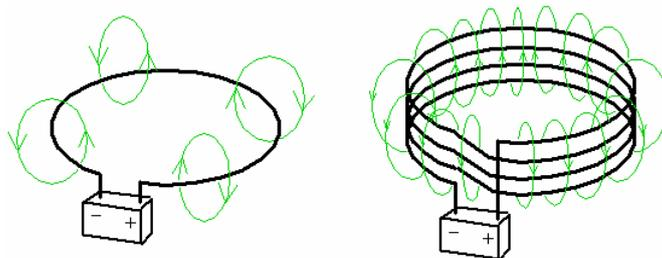
The left-side picture shows a wire-loop connected to a battery. Green lines depict the magnetic field generated by the wire loop (a simplified depiction). Note that inside the wire-loop, magnetic-field lines all point in the same direction. That is, if you look at the surface bounded (encircled) by the wire loop, you can see that a non-zero magnetic flux passes through that surface.
